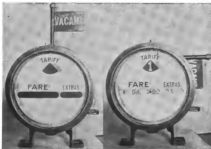
"DISENGAGED" AND "ENGAGED" VIEWS OF TAXIMETER.
